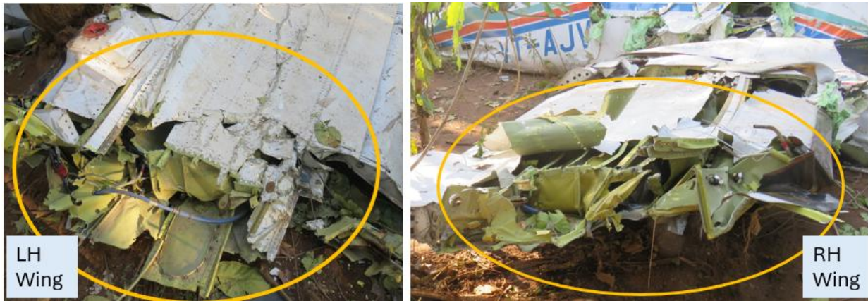
Figure 3: Damaged LH and RH Wing
