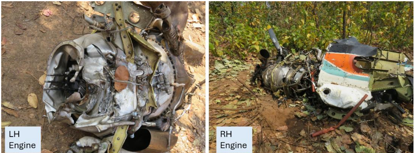
Figure 6: Damaged LH and RH Engines
